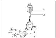
1. Drill chuck assembly 2. Chuck adapter
